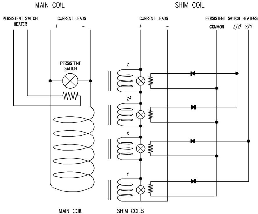
When the CS-4 Shim Supply Option is activated, the CS-4 uses its main current outputs to set the shim coil current. In shim mode the supply is software limited to a maximum current output. The current limit for each shim, the persistent switch heater current for each shim, and its overall status (enabled or disabled) is controlled through the menu system via the front panel keys.
