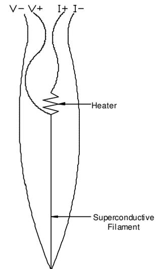
Sensors operating in a 3-wire configuration typically combine the leads I- and V- into a single lead. Doing so adds some lead resistance to the liquid level measurement that would show up as errors in the reading in most helium level monitors. The LM-500, however, has provisions for subtracting out lead resistance in 3-wire sensing systems.
