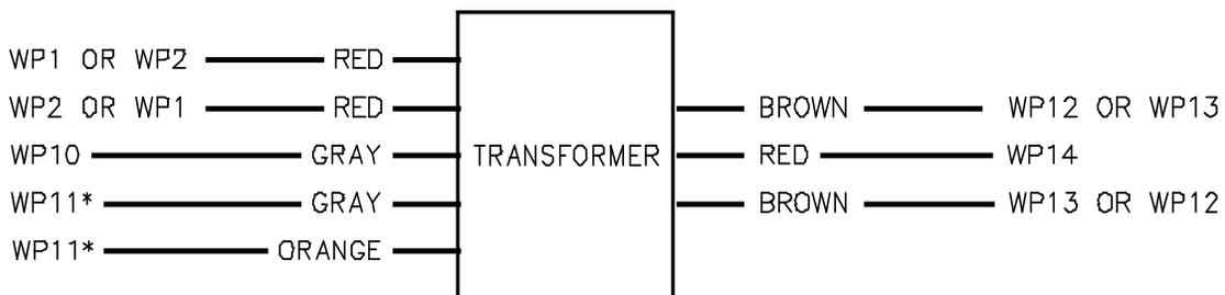
\* For almost all configurations of the LM-500, the gray connection to WP11 is used and the orange lead is not connected. The orange lead is connected to WP11 instead of the gray ONLY if the unit is to be used with 100V/50Hz or 200V/50Hz power AND with liquid helium level sensors having an active sensing length of more than 80 cm.
